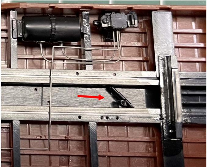
11. Locate and Install Brake Line. Referring to the photo locate the two halves of the brake line. Be extremely careful when removing these parts from the sprue as they are easily broken.
