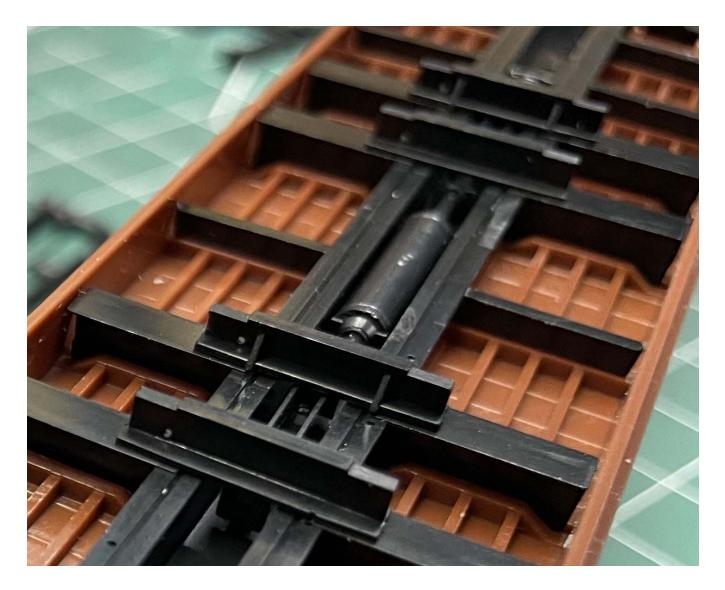
7. Locate and Install Reservoir Piping: From the wire parts bag locate the two U shaped wires for the reservoir piping. They will go from the reservoir to the bottom two holes of the AB valve, with the shorter "leg" going in the reservoir and the longer into the AB. Secure in the reservoir with CA but not at the AB valve yet to ensure you don't block the other holes.
