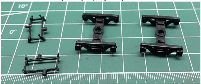
Install the brake shoe/cylinder by snapping the clips over the truck bolster.
