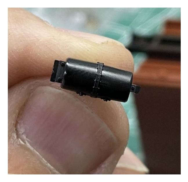
It has a pin that fits in a hole in the floor between the last set of crossmembers next to the bolster. Using a #80 drill open the holes in the reservoir to allow the wire parts to fit properly. Insert the post into the hole ensuring that it is resting on the crossmembers. Glue in place.
