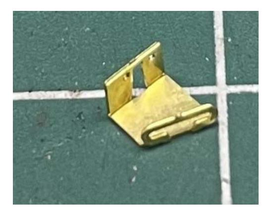
Install at the corner of the end by sliding the slot over the tab so that the flat part sits flush against the end of the car. Secure with CA.
