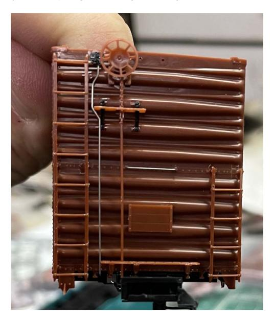
9. Locate and Install Cut Lever Bracket: From the wire parts bag locate the cut lever bracket. It is a brass etching that has a slot and a bend break. At the break, make a 90 degree bend as shown in the photo.
