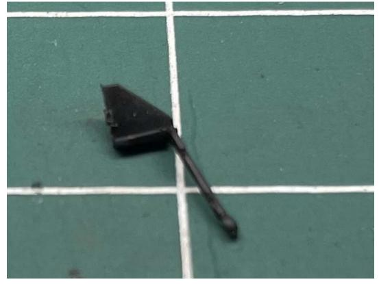
Position it so the tab fits in the notch and the bracket is lined up with the side of the pocket vertically. Secure with CA, again being careful not to glue the cover on. Also, attach the end of the air hose line to the bottom of the bracket with CA.
