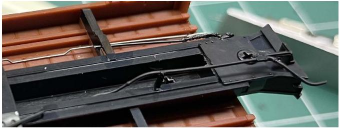
21. Locate and Install : The angle cock and air hose is a rubber part (see photo). It has a small tab that fits into a notch on the side of the coupler box.
