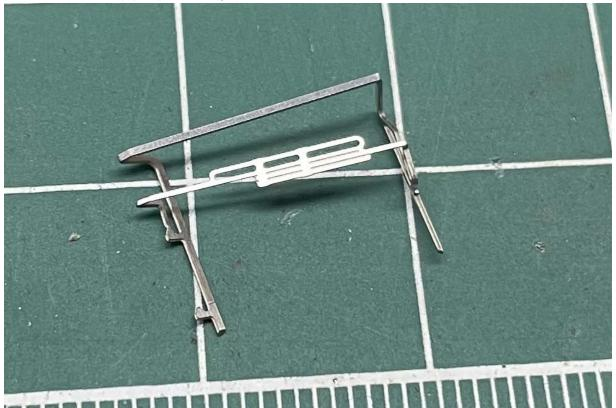
Feed the handle through the loop in the bracket and insert the other end into the hole at the edge of the coupler box cover (you may need to bend the end slightly to get it to fit properly). Tack the end at the cover with CA but leave the handle end loose to allow the installation of couplers.
