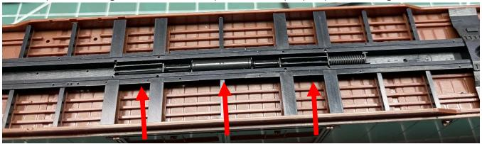
4. Locate, Choose and Install Reservoir: There are three different reservoirs to choose from. Refer to the photo to help identify the proper one for this version of the car.
