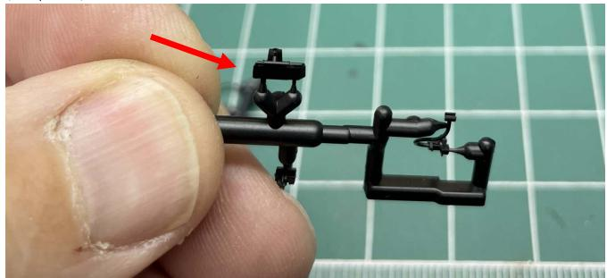
This part will fit into holes in the floor between the center sill. The pins are different sizes so it can only fit one way but see the photo of the part installed to ensure proper placement.
