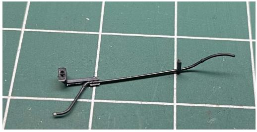
These parts fit into the rear hole in the cover and into a slot in the center sill. To make the installation go a bit smoother open the rear hole with a #70 drill. Position the part as shown and glue in place being careful not to glue the cover to the pocket.
