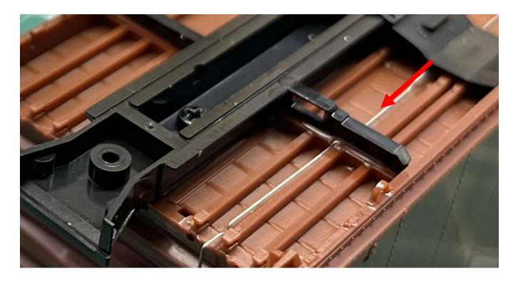
18. Locate and Install Brake Fulcrum: There are two different fulcrums to choose from. For this build we will use the one that has small flat spots on either side to the tip.
