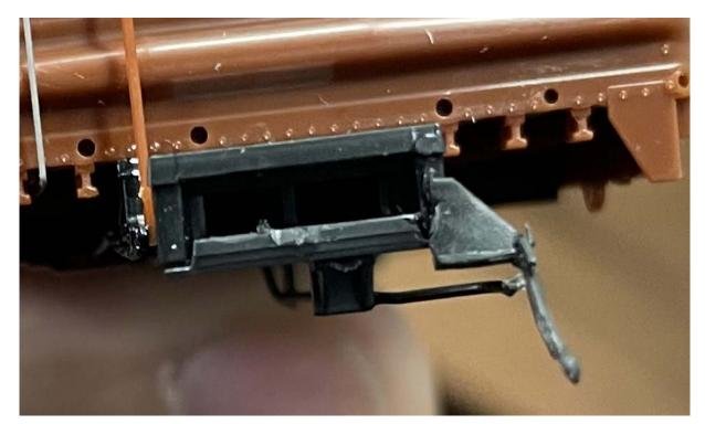
22. Locate and Install Bleed Rod: From the wire parts bag locate the parts for the bleed rod. There is a long wire piece, a small eyelet, and two brass guides - one short and one long.
