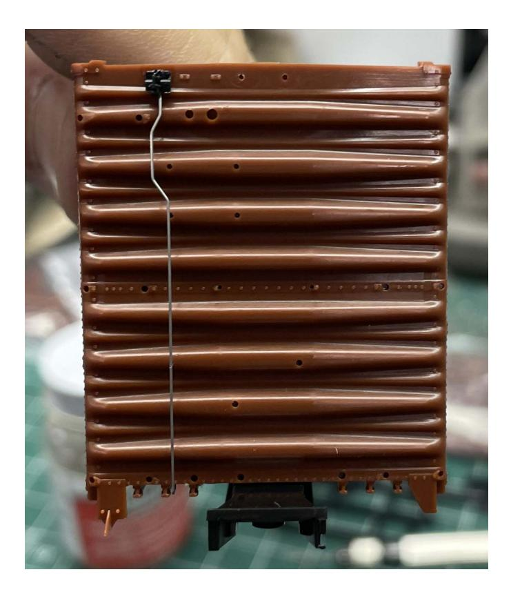
16. Locate and Install Underframe Retainer Line: The second half of the retainer line is also located in the wire parts bag (see photo). The part with the 90 degree bend goes into the hole with the first part of the retainer line and it fits in a slot in the floor next to the bolster. The end of the wire fits in a slot in the bolster itself. When positioned use CA to secure in the hole in the floor but not at the bolster to allow placement of the next part.
