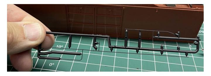
Also, try to remove as much flash from the attachment points to allow it to pass through the holes in the sill braces.
