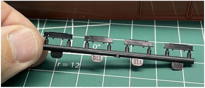
To make it easier to feed the piping through open the holes with a #77 drill. They have posts on the bottom that fit in holes in the center sill and also have small gussets on one side.
