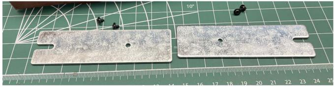
Set the weights in place and secure them with the four panhead screws from the wire parts bag.
