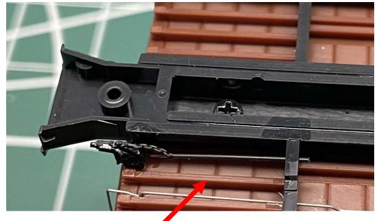
19. Install Coupler Box Covers: There are two different coupler box covers. The one we need for this version is the one that has the two holes at the edge of the cover slightly offset. There may be two small mold pins on the back edge of the coupler pockets that will need to be trimmed off to allow the covers to sit properly.
