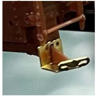
10. Locate and Install Cut Lever: There are two different cut levers included. See the photo for the appropriate style for this build.
