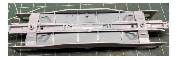
3. The shorter air line has one side that has a slight offset-this goes toward the B end. Put in position and glue in place.
