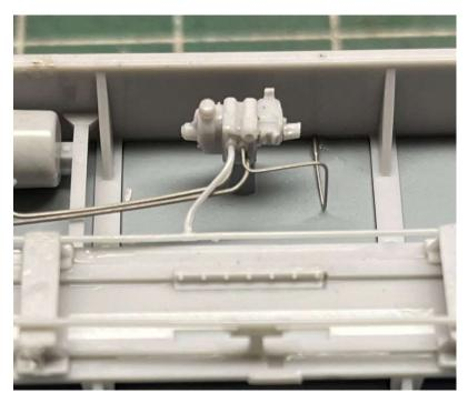
12. **Install Dirt Collector Pipe:** The dirt collector pipe (see photo) rests on the train line and fits into the last opening in the AB valve. Once this part is in place you can secure all parts in the AB valve.
