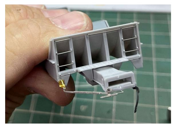
32. **Install Car Body Grabs:** There are four grab irons on the carbody, one at each corner of the sides. Use four of the remaining eight short grabs for these. Secure with CA.
