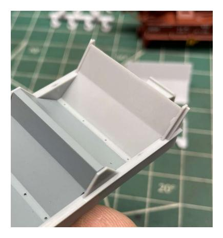
21. **Install End Cages:** There are two end cages, one for the A end and one for the B end. They sit inside the car sides and rest on the center sill and against the end slope sheet. Position each end and glue in place, making sure you put the right cage on the right end of the car. (the B end is the one closest to the reservoir).
