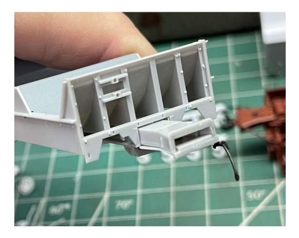
22. **Install Fulcrum:** On the B end, there is a small slot in the bottom of the end cage. This is for the fulcrum. Position the fulcrum by inserting the tab into the slot and glue in place.
