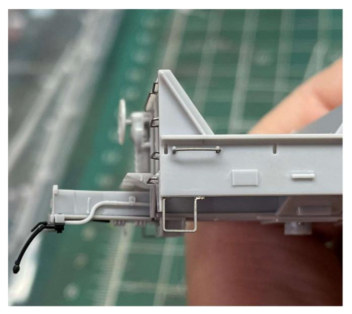
34. **Install Hood Cover Holders/Guides:** The last two parts for the carbody are the hood cover holders/guides. They have tabs that fit into slots on the top of the sides of the car. Position on each side and glue
