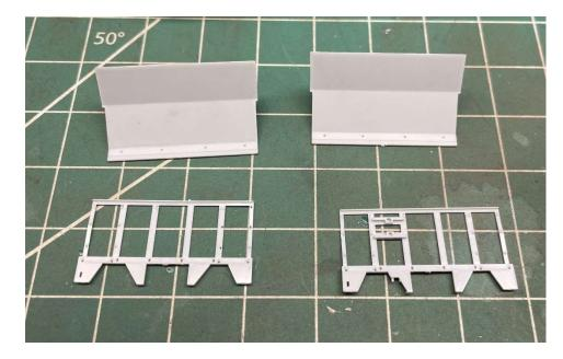
20. **Install End Slope Sheets:** The end slope sheets have a small lip on the lower end that fits underneath the floor. Position it under the floor and seat it until the two center supports rest on the center sill and the sides rest on the raised ridges of the car sides (see photos). Glue in place.
