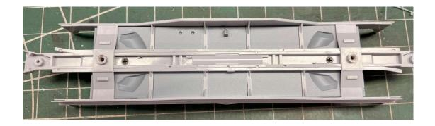
2. Install Train Lines: Position the longer train line so that the 90-degree bend is toward the right. The casting has tabs that fit into holes in the center sill to aid in locating. Set in place and secure. It may not be straight but when other parts are added later it will straighten itself out.
