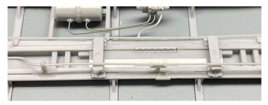
10. Install Retainer Valve Line: Locate the retainer valve wire (see photo). The short leg goes into the opening in the AB valve just above the right-hand reservoir wire and the long end rests on the floor in a small slot next to the car side. This part is a bit tricky to set in place so to make it a bit easier use a small bit of CA to tack the longer leg in place while you position the short leg in the AB valve. Again, do not use any glue at the AB valve yet.
