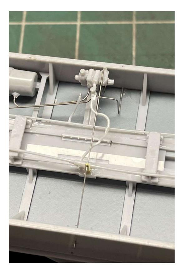
16. Install Coupler Cushion Guides: There are two cushion guides that fit at the back side of the coupler box. They also have two tabs that fit into slots in the center sill. They have a slightly trapezoidal shape and the longer side faces the ends of the car. Set in place and secure.
