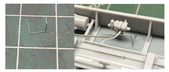
11. Place Air Line/AB Valve Connection: The short leg coming off the train line goes into the opening on the left hand side of the AB valve above the left reservoir wire. Insert but do not glue.
