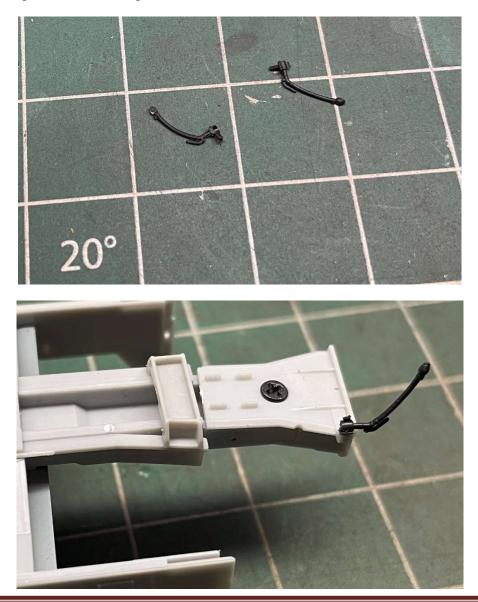
19. Install Air Hose Pipes: Locate the two air hose pipes. These parts have small pins that fit into holes in the side of the coupler box. The tail end fits in the slot between the coupler box and center sill. You may need to trim a little bit off the back end of the pipe so it fits properly. The other end of the pipe fits into the back side of the air hose. If you haven't added couplers yet, do not glue the pipe to the air hose as you will need to be able to get the coupler box cover off.
