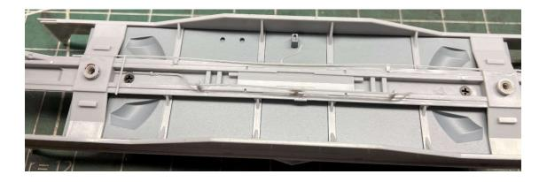
4. Install Center Sill Cross Braces: Locate the two center sill cross braces. They have small tabs that fit into slots in the center sill. Set these in place and glue. (after these are installed, the train lines should be now be straight)
