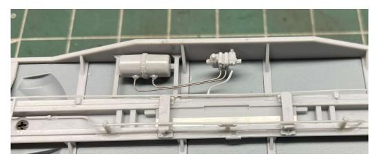
9. Install L Brackets: There are two L brackets that fit into slots on either side of the center sill. The bottom part of the L rests in the slot and faces the center of the car. Glue both parts in place.
