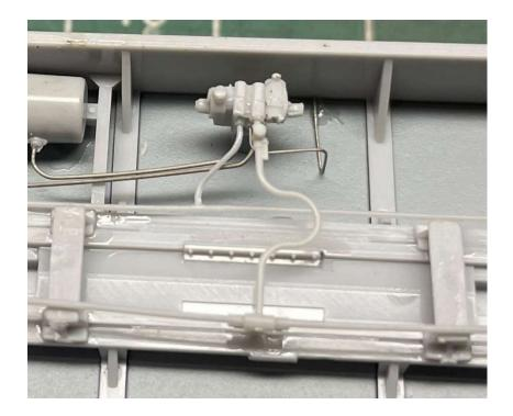
13. **Install Bleed Rod Assembly:** The bleed rod assembly has three parts- a long and short wire and a brass standoff. Locate the parts (see photo) and install the standoff in the slot in the center sill next to the support for the dirt collector pipe. Position it so the bottom of the L faces the center of the car. Secure with CA.
