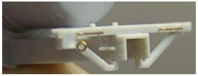
31. **Install the coupler lift bars.** Insert the cut levers through the eyebolts and into the small hole on the bottom of the coupler box cover. If you have not installed the couplers yet, just tack the cut lever in place at the coupler box so that it can be removed to install the couplers after painting.
