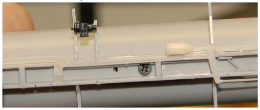
13. **Install the air reservoir**. The air reservoir (part 16) has three mounting legs that have tabs that fit into holes in the center sill. The two air lines coming out of it fit into the two bottom holes in the triple valve (the ones closest to the tank body). Glue assembly in place.
