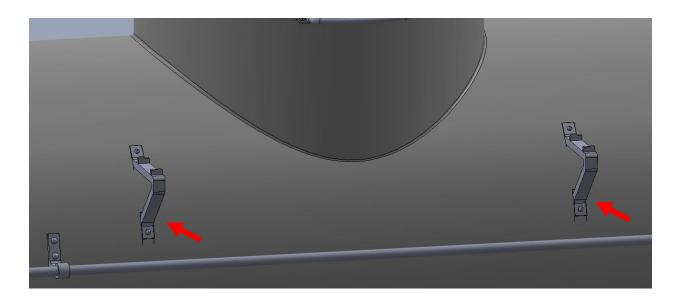
36. **Assemble the side platforms.** Locate the etched metal platform parts. Install the last two grab irons into the bottom. Install them so they project outward from the platform and are vertical. Glue in place with CA.
