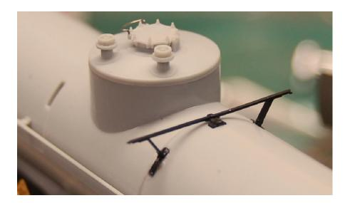
46. **Install the dome platform railing and ladder assembly.** The platform railing/ladder assemblies have small notches on them that fit the corners of the platform supports. Glue at the corners of the platform, and also insert the locating pins on the bottom of the ladders into the holes of the walkway. Glue the ladders to the walkway with CA. Repeat on other side.
