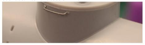
21. **Install the dome vents and cover.** All are keyed for placement, glue in place when installed.
