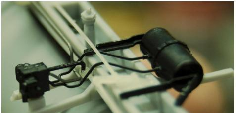
17. **Install the largest drop grab irons – the brake hangars.** Locate the three largest drop style grab irons from the wire parts bag. These will fit into holes in the center sill by the levers.
