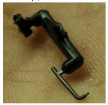
It fits into the remaining hole in the triple valve and a small locating tab in the train line. Glue in place.
