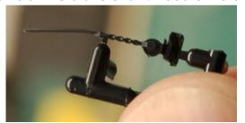
The brake chain has two pins that fit into the two outer holes in the end sill. Mount this part on the underside of the sill with the end of the chain fitting into a small hole in the bolster face. Glue in place.
