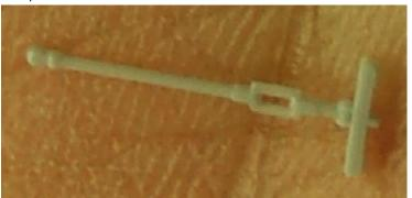
Each of the four tank straps has a long end and a short end. The short end goes into a hole in the top of the bolster located right behind the walkway. The long end fits into the slot in the strap anchor. Insert the short end into the hole in the bolster and rest the long end of the strap into the slot in the strap anchor with the end to the strap fitting all the way to the top of the slot. Secure with CA being careful not to fill the slot with glue. Repeat this process for all four.
