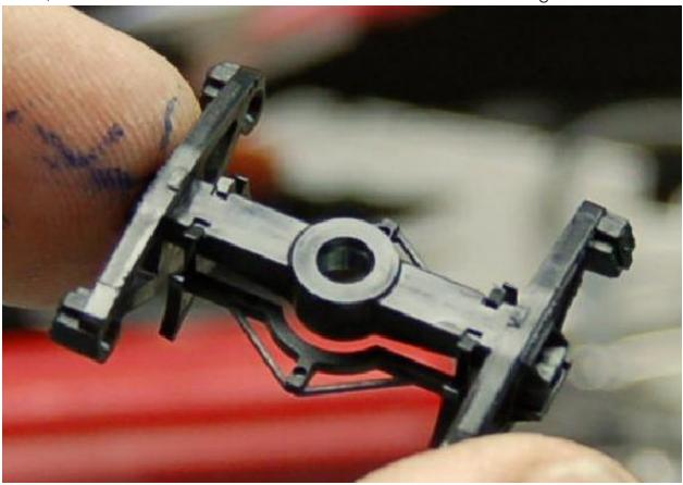
33. Install end tank rail brackets. Locate the two end tank rail brackets (in bag 18).
