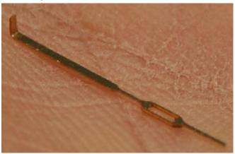
41. Attach the tank straps to the tank and underframe. Insert the straight end of the strap into the hole in the bolster and the bent end into the hole in the side of the tank. Secure both ends with CA. Repeat this process for all four tank straps.
