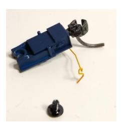
2. Carefully remove the coupler box. (gently wiggle it out)
