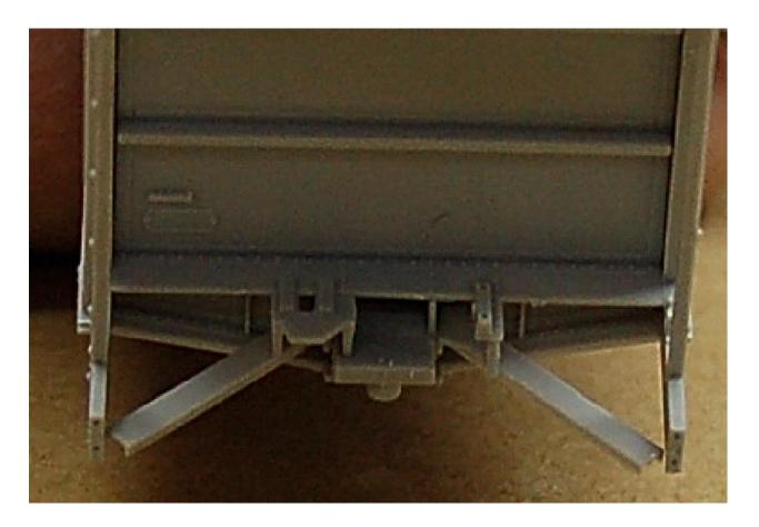
11. **Install the air reservoir.** Start the installation of the brake components by installing the air reservoir. It sits on the bracket that is on top of the side sill and the post on the channel installed in the previous step. The small holes in the reservoir face the end of the car. Glue in place.
