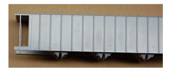
3. **Install the End sheets into the body assembly.** Start with the end sheets. There is an A end and a B end (the B end is the brakewheel end). The B end sheet has a small casting that looks like a plate with a bar over it in the lower left corner (pictured here).
