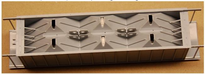
6. **Install the cross braces.** There are two large cross braces that fit over the triangular gussets. Slide the cross braces over the gussets and seat so that the top of the cross brace sits slightly below the side of the car. Glue in place.
