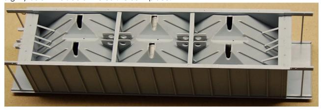
7. **Install bolster parts.** The bolsters have a small tab on them in the center of the casting. This tab faces the end of the car. You will also see small notches in the car sides that the ends of the bolsters fit into. There are also small pins on the slope supports from the previous step that aid in the positioning of the bolsters. Position bolsters and glue in place making sure that the ends of the bolsters fit flush with the car side when seated in the notches. Glue in place.
