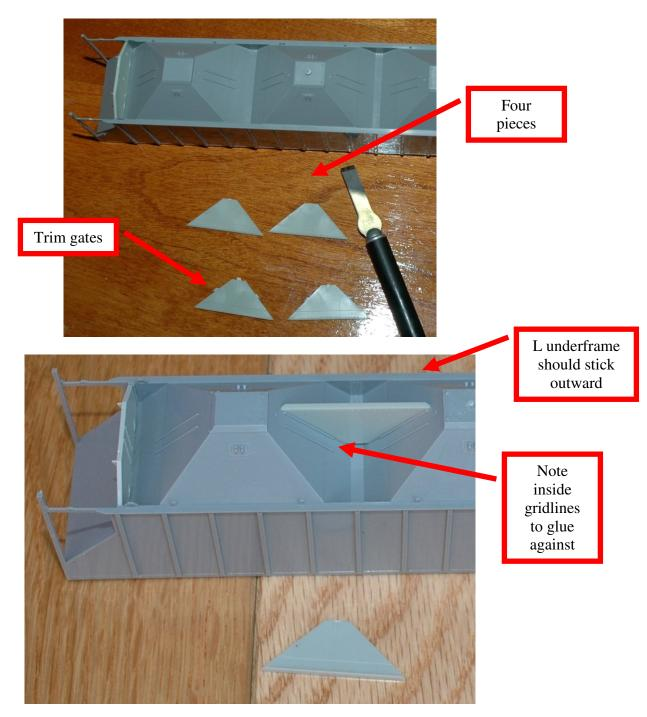
6. **Install the 4 centersill crossmembers.** These install perpendicular to the carbody side and the centersill, fitting between each. Prototypes built after October 1969 likely do not have these parts.
