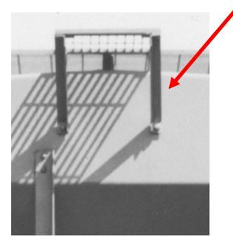
**27. Attach grab irons to the Roofwalk:** Attach the supplied wire straight grabirons to the holes in the roofwalk. Drill a hole through the roofwalk so that the 18" grabiron is positioned halfway between the angle of the roofwalk. The grab iron should have a roughly 30 degree bend in it to match the slope of the roofwalk. Photo:
