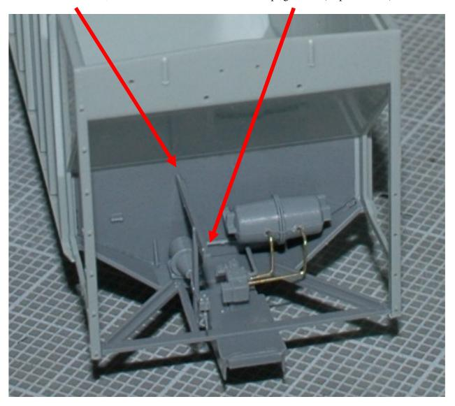
**13. Attach the A end uprights:** Using sprue nippers, carefully degate and clean the A end uprights found in the small end uprights sprue. Cut the tops of the end uprights square using sprue nippers. Test fit on A end, and then cement so that the uprights fit into the holes at the top and directly between the end uprights molded into the body. It should also sit right on top of the coupler box in the center. (See photo in step 14 of B end upright installation for guidance).
