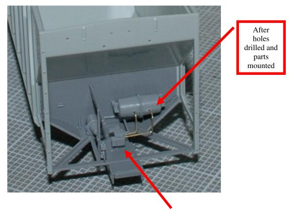
11. Attach the AB valve: Degate and clean the AB Valve part from the small brake parts part sprue. It mounts on top of the small "box" in the B end, and its air line runs toward the slope sheet (simulated to attach to the back side of the brake cylinder in the next step). If you elected to add the air line from the air reservoir in the previous step, it is advised that you drill holes in the AB valve at this point and test fit the wire parts before attaching it.
