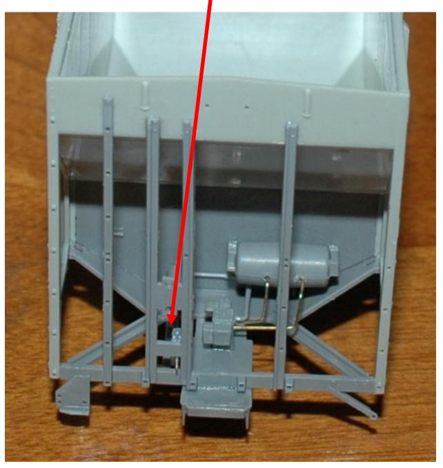
**15. Attach the brakewheel housing:** Degate the brakewheel housing from the small brake parts part sprue. Attach to the B end, on top of the mounting plate that has the two holes in it. Slide the part into position so that the bottom U shaped part slips over the clevis part.
