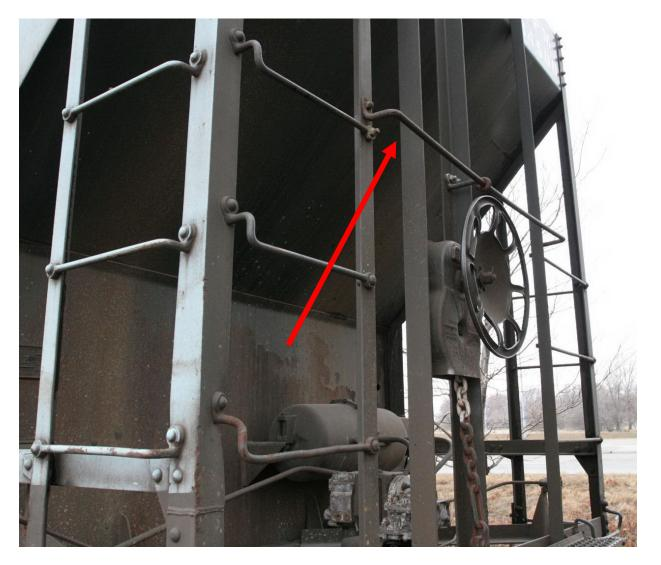
**21.** Attach wire grabirons to non-ladder side of end: Using either .012" wire or brass, bend grabirons to fit between the rightmost ladder upright and the corner posts. Each end requires three of these.
