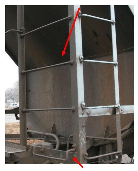
**22.** Attach wire drop grabiron on each end: Using supplied drop grabirons, place one drop grabiron in each end of the car in the lower right corner of the horizontal end runner. There is one hole here on the end, located just above the 45 degree angle support for the stirrup step. The left hole needs in the model needs to be hand drilled out.
