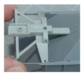
8. Attach bolster plates: Degate and clean the two bolster plate parts. These need to be cleaned especially well on the sides because this signature part is visible above the trucks of the car. The parts should be mounted so the hole for the truck screw lines up with the hole in the coupler bolster, from step 7 above. Note the small ridge in the plastic that helps to locate this part on the car. The long tab "points" toward the coupler box.
