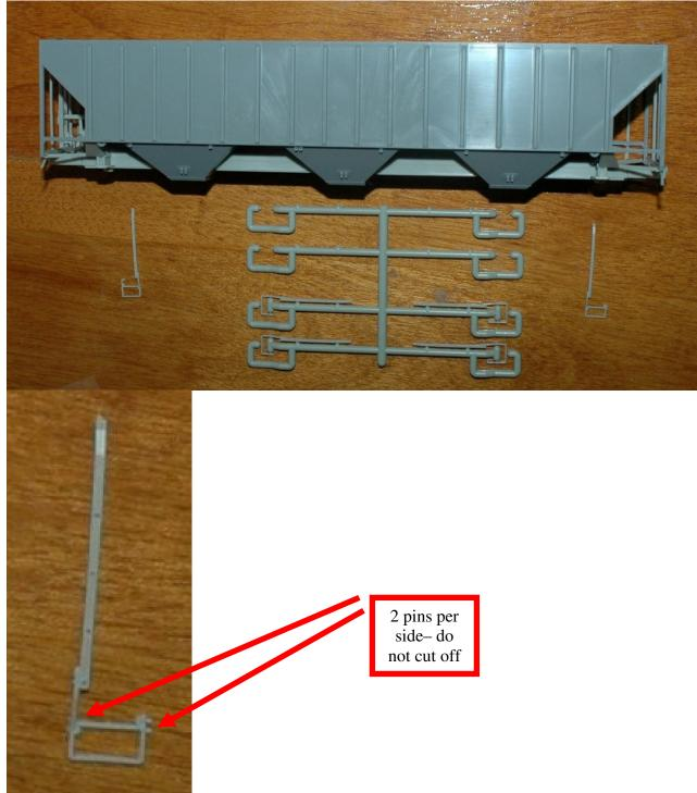
**17. Attach the Brake Line:** Using sprue nippers, degate and clean the 2 parts that form the brake line. These parts are located in the end upright part sprue. The part that has 3 supports goes on the left side of the car, whereas the part with the 4 supports goes on the right side.
