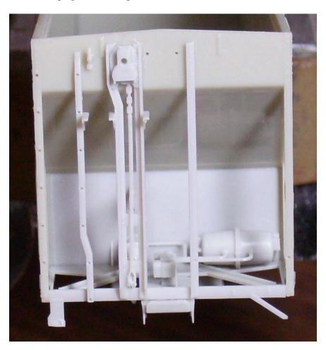
10. **Attach the A end uprights:** Using sprue nippers, carefully degate and clean the A end uprights found on the "End frames" sprue. Cut the tops of the end uprights square using sprue nippers. Test fit on A end, and then cement so that the uprights fit into the holes at the top and directly between the end uprights molded into the body. It should also sit right on top of the coupler box in the center. (See photo in step 11 of B end upright installation for guidance).
