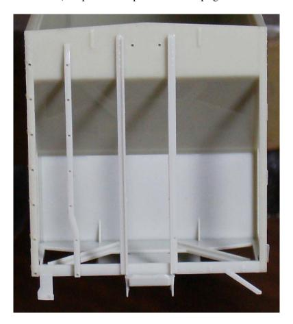
11. **Attach the B end uprights:** Repeat the process highlighted above, this time on the B end. Note that the clevis fits between the uprights and the horizontal member cements to the backside of the upright. Some slight trimming of the clevis have be required so it sits against the
