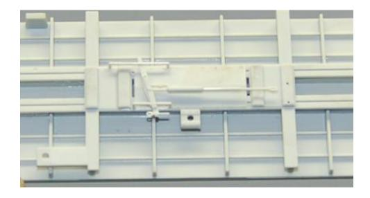
13. **Install the underbody brake appliances.** Locate the reservoir, AB valve, and cylinder and open the holes with a #79 drill. Position the parts as shown in the photo making sure the holes in the AB valve are facing toward the center sill of the car. Shorten the rod behind the chain on the lever assembly so that it fits flush with the end of the cylinder.
