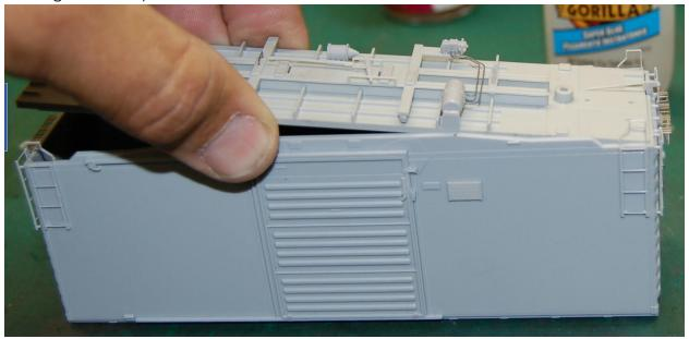
18. **Install the retainer release valve**. This plastic part should be attached in line with the cross member closest to the AB valve and glues to the underside of the side sill. You may need to shorten the mounting tab slightly so that it fits flush.
