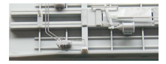
20. **Install the air line from the brake cylinder to the AB valve.** Insert the wire from the brake cylinder to the AB valve and secure with CA at both the cylinder and the AB valve, also securing all other wires at this time.
