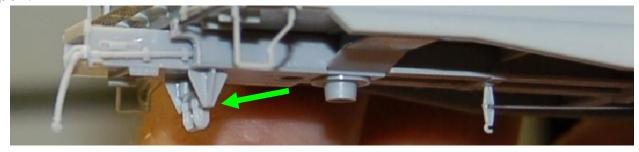
27. **Select the correct coupler lift bars.** This Tangent kit provides you with two different coupler lift bar parts to choose from. Choose which you will use based on your prototype. This is the version applied to the cars built for Illinois Central:
