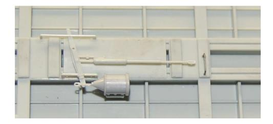
15. **Install the slack adjusters.** Install the two small plastic slack adjusters into the small holes by each bolster, orienting them so that the slot faces the center of the car.
