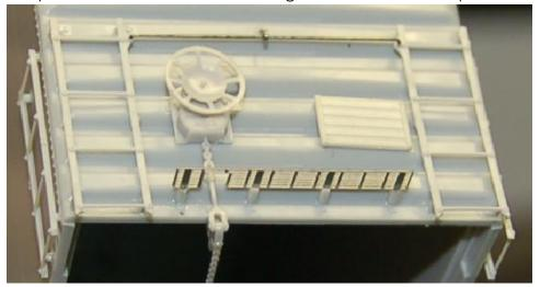
9. **Install the stirrup steps.** The last step in the body assembly is the four stirrups. They fit into notches inside the side sills of the carbody. If you look at the stirrup you will notice that the mounting tabs are slightly offset.
