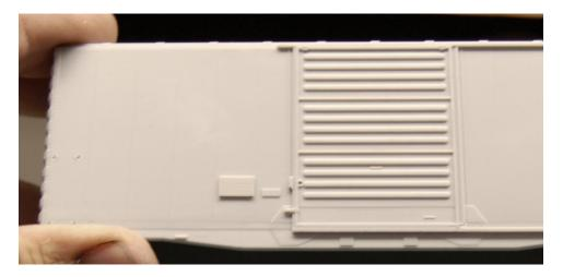
2. **Install the door levers.** Just below the tackboards on the sprue are the door levers. These go on the left hand side of the doors. Mount them so that they are pointing straight down and glue in place.
