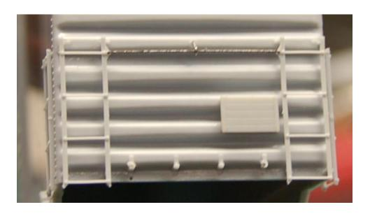
7. **Install the brake parts.** The B (brakewheel) end of the car has extra mounting holes for the brake gear. Very carefully de-sprue the brakewheel housing and chain casting and glue in place. Again, very carefully de-sprue the fulcrum and chain assembly and glue in place on the end of the car aligning it with the chain from the brakewheel housing. Glue the brakewheel into the brakewheel housing.
