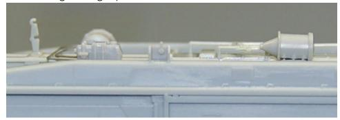
19. **Install the retainer air line.** After the glue has set, locate the "C" shaped wire and install it from the bracket to the center hole of the AB valve. The longer leg of the wire goes into the bracket and the shorter goes into the AB. Secure with CA at the bracket but not the AB valve.
